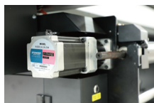
High quality DC servo motor: good stability and long service life;
