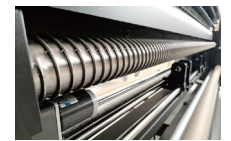
Adopting a spiral roller feeding system for smoother material feeding
