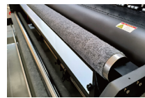
Configure a soft film tension system to meet the pressure requirements of different materials
