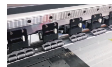
3 independent adjustable lifting and lowering wheels
