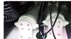
Electrostatic brush Eliminate static electricity, improve printing quality, and eliminate fire hazards.
