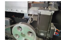
High quality DC servo motor with good stability and long life.
